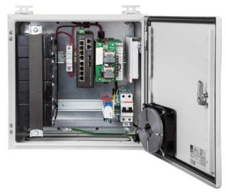
The NSBox access Node is a completed product for installation and operation in any climates, which is immediately switched on in the operating mode. The device has one 110-220VAC external power line, up to 16 Ethernet ports for connecting IP video cameras, wireless access points or other PoE equipment and up to 4 Uplink Ethernet for communication with another access nodes or an aggregation center.
