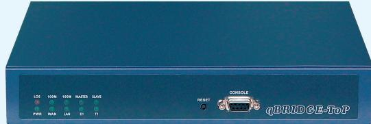
qBRIDGE-401 is a very reliable, high performance and cost effective converter/inverse multiplexer suitable to connect Fast Ethernet LANs over up to four bonded E1 channels. The qBRIDGE-401 devices support four framed E1 ports. It also has embedded four ports 10/100Base-TX Ethernet switch with enhanced QoS and traffic prioritization support. Device can be used in Ethernet over PDH/SDH or point-to-point applications.
